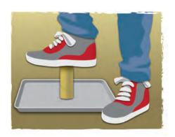
you make the second column stronger, using only tape and sand? Make a prediction, then repeat step 2.
